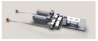
All systems can drive various kinds of propulsors, e.g. FPP, CPP, WJ, Voith Schneider, also in combination with CODAD, CODOG, CODAG, COGAG, CODELAG hybrid-drives.
