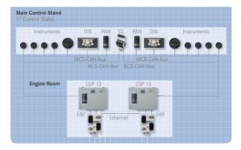
Simple interfaces connect the Monitoring & Control System BlueVision | NewGeneration with the MTU diesel engine (via EIM) and the gearbox.
